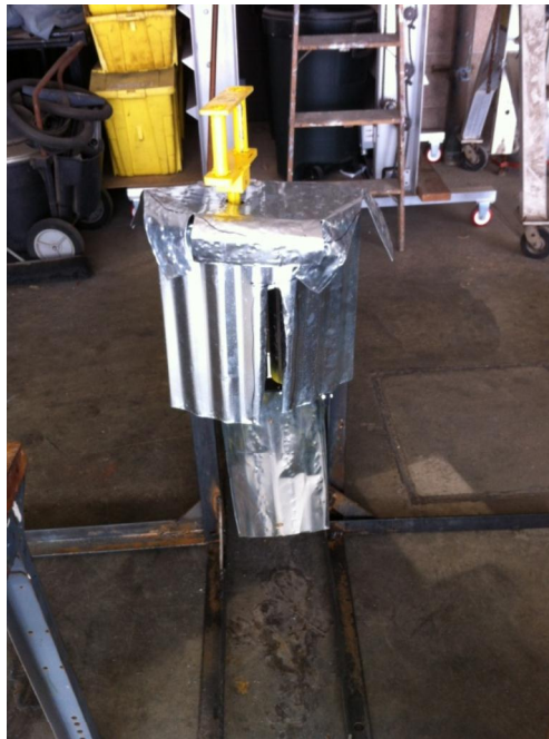
Figure 11 ñ Safety Shroud and Funnel Installed on Press
